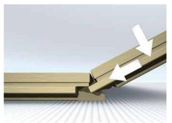
Hold the panel to be installed at an angle of 20° to 30°. Move the panel gently up and down and at the same time exert forward pressure. The panels will automatically click into place.
